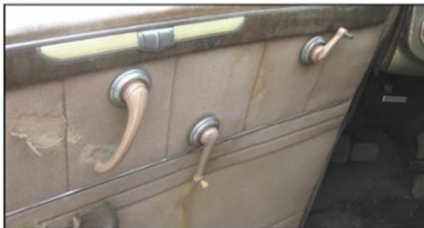
This 1942 Special has the rare, plastic, door and window crank handles—a late 1942 change, due to the W.W.II restrictions on chrome-plated parts.
