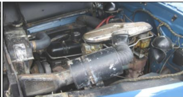
Compound carburetors were optional on the Specials in 1941 and 1942, but this '42 had them. It also has the 1942-only silencer and hose mounted ahead of the air cleaner assembly.
